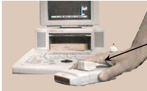
Ultrasound head with pcBIRD positioning system receiver mounted
